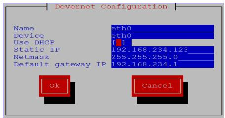
Provide all the required information such as IP Address, Netmask and Gateway Address. Click on OK
