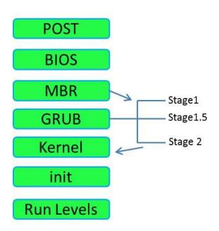
POST: Power on self-test - Hardware will check it self
