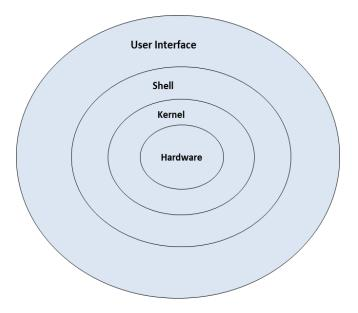
*Kernel:* It is a program. Kernel is a Core component of operating system, interacts directly with hardware and provides low level services to upper layer components.
